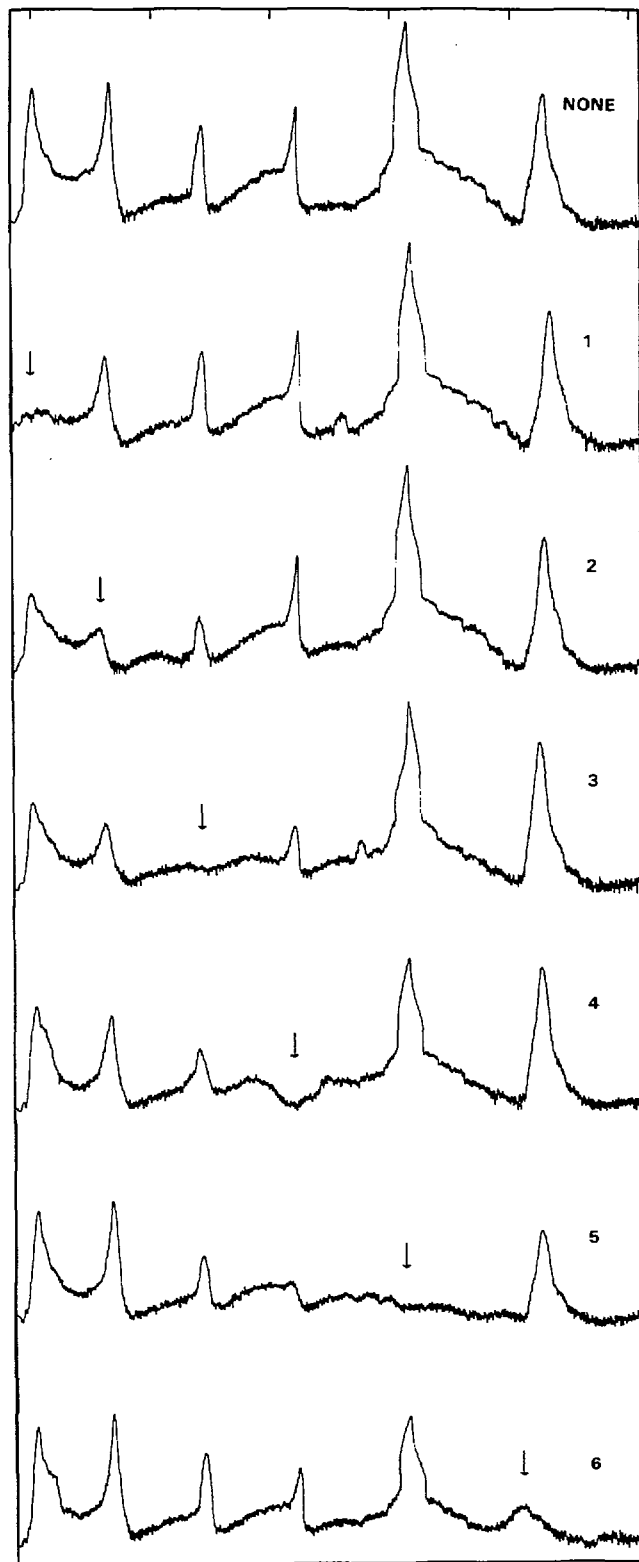
Fig. 12. Effect on side radiation of wrapping lossy material around feeder section of each cell in antenna #18. Numbers at right indicate which cell has been wrapped. Arrows indicate anomaly most strongly affected. Horizontal frequency scale is same as in foregoing figures.
