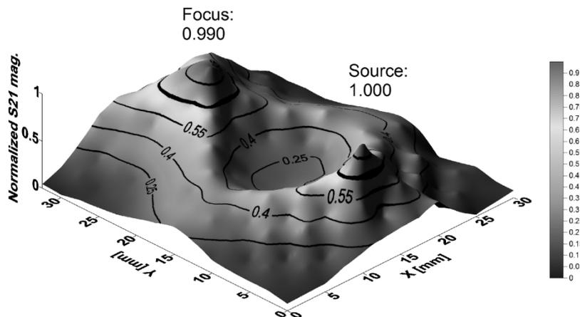
Fig. 8. Focusing measurements at 1.5 GHz. Heavy contour is at 0.707 of focal maximum of 0.990 (units of normalized  $|S_{21}|$ ).
