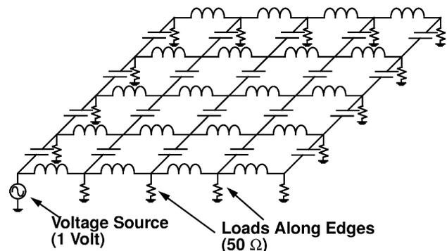
Fig. 2. Uniform anisotropic planar L-C grid over ground, with corner feed and resistive edge loading.
