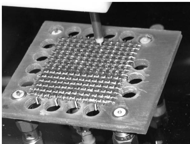
Fig. 4. Experimental setup showing a scanning open-ended probe over a nonuniform L-C grid with the transposed-element interface near the middle of the grid.
