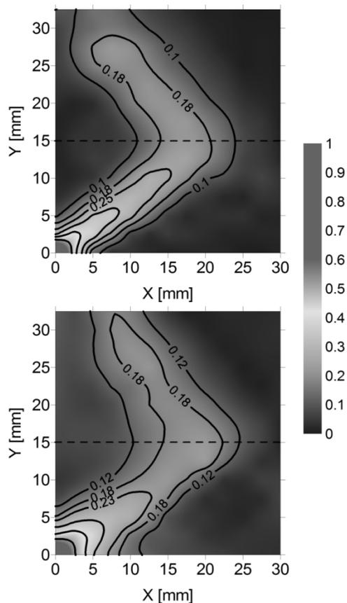
Fig. 5. Resonance-cone refraction at 1.2 GHz—simulation (top) showing contours of grid-to-ground voltage magnitude, and experiment (bottom) showing contours of normalized  $|S_{21}|$ . Refraction occurs at the  $y = 15$  mm interface between two grids with transposed (interchanged) L and C elements.
