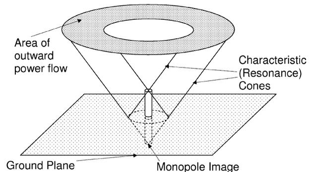
Fig. 1. Monopole antenna in highly anisotropic (resonant) plasma, showing characteristic cones (resonance cones) extending from antenna ends.
