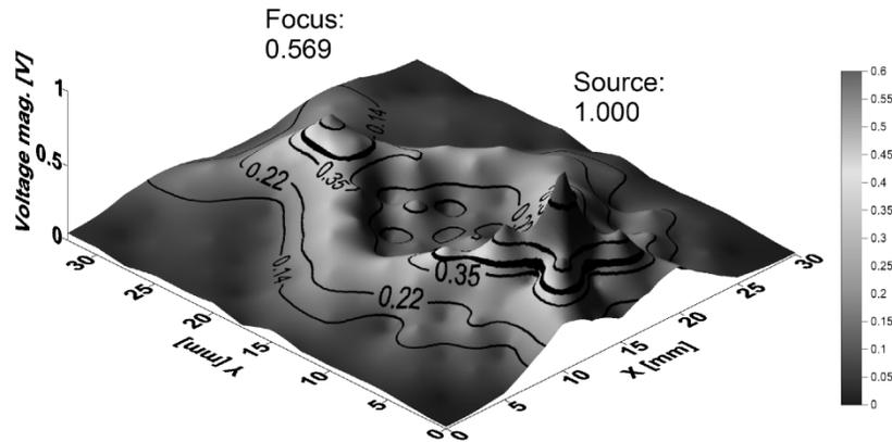
Fig. 6. Focusing simulation at 1.5 GHz. Heavy contour is at 0.707 of focal maximum of 0.569 V.
