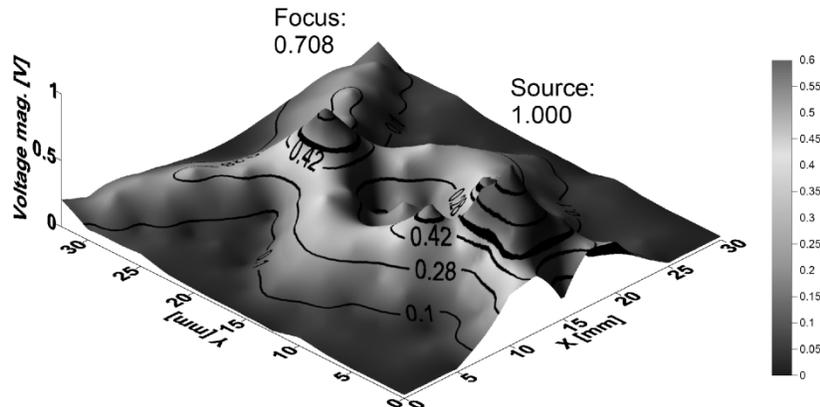
Fig. 7. Focusing simulation results at 1.7 GHz. Heavy contour is at 0.707 of focal maximum of 0.708 V.
