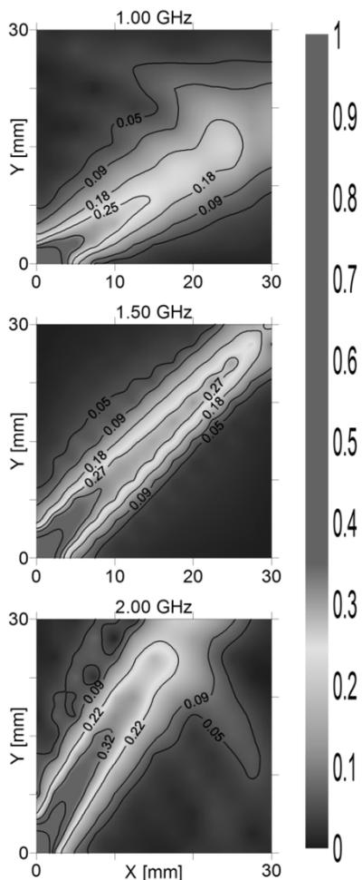
Fig. 3. Uniform-grid moment-method simulation displaying resonance cones at three frequencies. Contours show grid-to-ground voltages.
