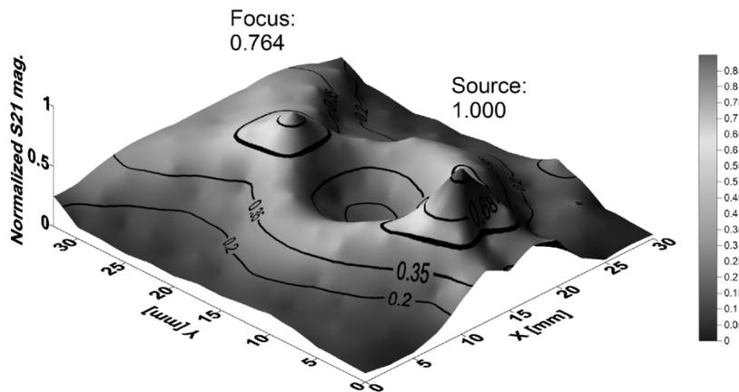
Fig. 9. Focusing measurements at 1.7 GHz. Heavy contour is at 0.707 of focal maximum of 0.764 (units of normalized  $|S_{21}|$ ).
