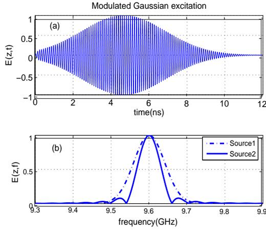
Figure 3. (a) Modulated Gaussian excitation with enforced front (b) frequency distribution of the Gaussian excitations with smooth front (source1) and with enforced front (source2)
