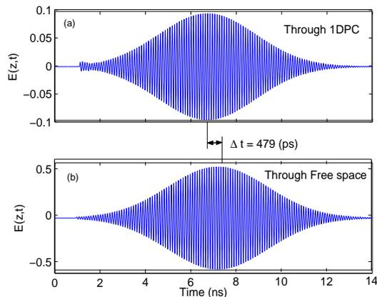
Figure 1. Pulse advancement in 5slab 1DPC.
