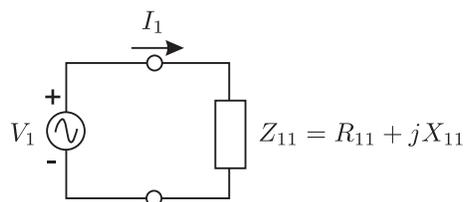
We now wish to use the equivalent circuit to help us predict the power delivered to a load attached to the receiving antenna when the other antenna is used to transmit a signal. Let's begin by using antenna 1 as the transmitting antenna and antenna 2 as the receiving antenna. We can model the transmitter as follows, if the receiver is located a large distance away. We terminate the receiving antenna in a load impedance  $Z_L$  which represents the input impedance to the receiver
