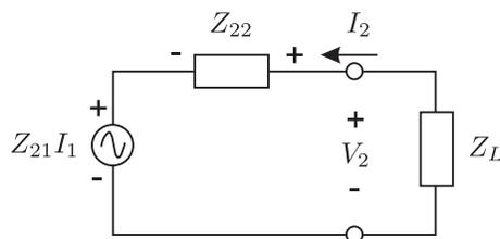
For maximum power transfer to  $Z_L$ , a *conjugate matching condition* must exist. That is,
