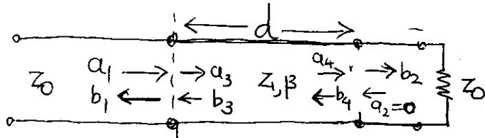
$$\text{We can write: } V_1 = \sqrt{Z_0} (a_1 + b_1) = \sqrt{Z_1} (a_3 + b_3) \quad (1)$$
