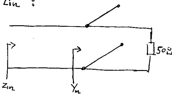
$$0.2e^{j10^\circ} = \frac{Z_{in} - 50}{Z_{in} + 50} \Rightarrow Z_{in} = 50 \frac{S_{11} + 1}{1 - S_{11}} = \frac{50(1 + 0.2e^{j10^\circ})}{(1 - 0.2e^{j10^\circ})} = 41.25 + 16.35j$$
