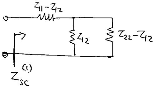
$$Z_{sc}^{(1)} = Z_{11} - Z_{12} + \frac{Z_{12}(Z_{22} - Z_{12})}{Z_{22}} = Z_{11} - \frac{Z_{12}^2}{Z_{22}} \quad \dots \quad (1)$$
