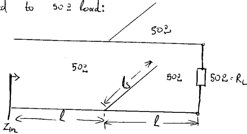
$$\text{Then } S_{11} = \Gamma_{in} = \frac{Z_{in} - 50}{Z_{in} + 50} \quad \dots \quad \dots \quad \dots \quad (5)$$
