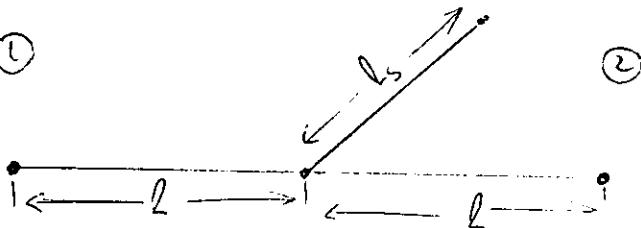
The stub provides the magnitude of  $S_{11}$  and the line its phase.
