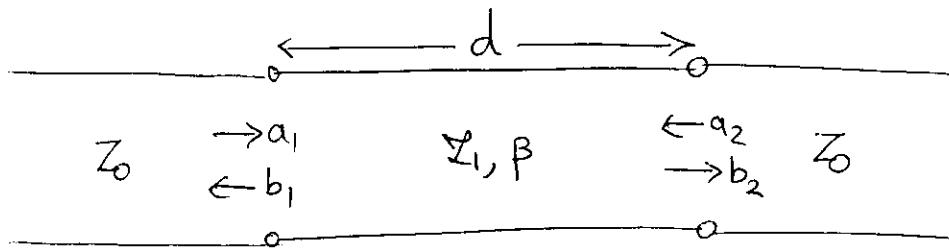
$$\begin{pmatrix} b_1 \\ b_2 \end{pmatrix} = \begin{pmatrix} S_{11} & S_{12} \\ S_{21} & S_{22} \end{pmatrix} \begin{pmatrix} a_1 \\ a_2 \end{pmatrix}$$
