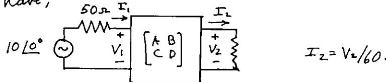
$$V_1 = AV_2 + BI_L = (A+B/60)V_2$$
