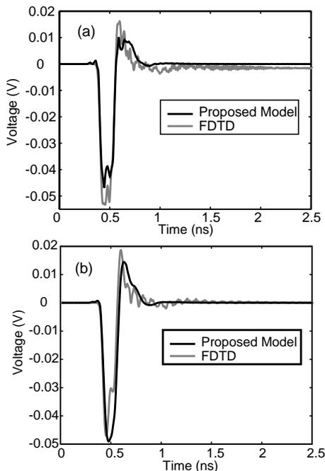
Fig. 3. Noise voltage between the parallel plates for differential vias,  $S=1 \text{ cm}$  and  $R=2 \text{ cm}$  (a) Top planes, (b) Bottom planes.
