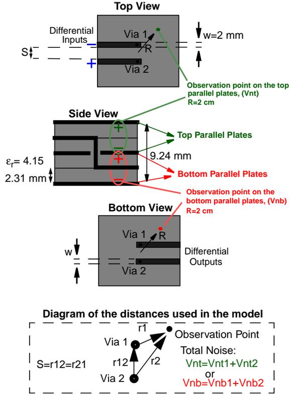
Fig. 1. Multilayer differential via structure.
