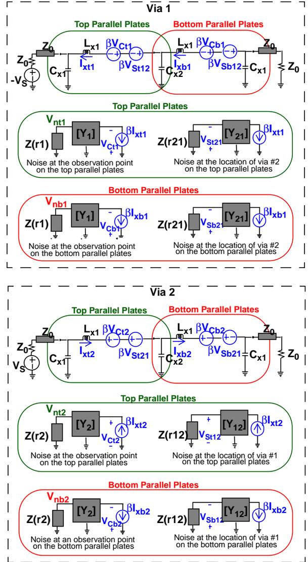
Fig. 2. Proposed equivalent circuit for the differential via configuration of Fig. 1.
