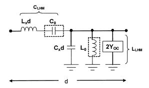
Fig. 8. 1-D unit cell of Fig. 6 with the effect of the transverse host medium represented as a shunt capacitance  $Y_{\rm OC}$ .
