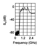
Fig. 14. Experimentally obtained frequency response of a 1-D LHM structure; six cells of size 5 mm each.
