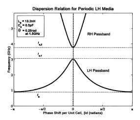
Fig. 5. Dispersion relation for periodically L-C loaded LHM using  $L_0=13.2$  nH,  $C_0=0.5$  pF, and  $\theta=0.25$  rad at 1.5 GHz, indicating Bragg frequency  $f_b$  and stopband limits  $f_{C,1}$  and  $f_{C,2}$ .
