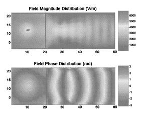
Fig. 13. Vertical electric-field distribution due to a voltage source illuminating the interface between an unloaded transmission-line grid (RHM with n=+2.25) and a dual L-C loaded grid (LHM designed for n=-5.5) with periodicity d=5 mm and relative permittivity of space  $\varepsilon_{\scriptscriptstyle T}=2.53$ ; The horizontal axis is labeled according to cell number.
