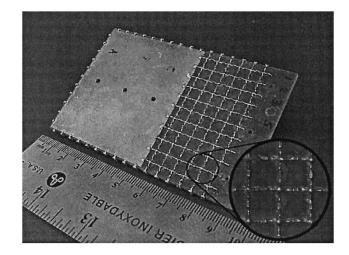
Fig. 15. Focusing device: LHM prototype interfaced with a parallel-plate waveguide ( $60 \text{ mm} \times 95 \text{ mm}$ ). The inset magnifies the surface of the LHM unit cell.
