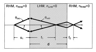
Fig. 3. Internal and external focusing using an LHM slab of thickness d.
