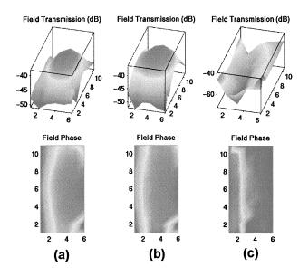
Fig. 17. Experimental data showing focal regions observed in the  $11 \times 6$  cell LHM at: (a) 1.55 and (b) 1.65 GHz (both within the LHM passband of Fig. 16) and (c) the lack thereof at 2.55 GHz (inside a stopband).
