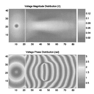
Fig. 12. Point source illuminating an RHM/LHM interface at 2 GHz (relative refractive index -2, finite air-filled transmission lines with  $d=5\,$  mm included in each unit cell), focusing observed in both phase and magnitude. The horizontal axis is labeled according to cell number.
