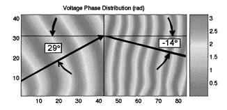
Fig. 9. Plane wave illuminating an RHM/LHM interface at 2 GHz (relative refractive index -2) at an incident angle of  $29^{\circ}$ . Refraction observed at  $-14^{\circ}$ . The horizontal axis is labeled according to cell number, and the right-hand-side vertical scale designates radians.
