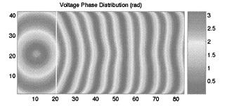
Fig. 10. Point source illuminating an RHM1/RHM2 interface at 2 GHz (relative refractive index +2, finite air-filled transmission lines with  $d=5\,$  mm included in each unit cell). No focusing was observed in either phase or magnitude. The horizontal axis is labeled according to cell number.
