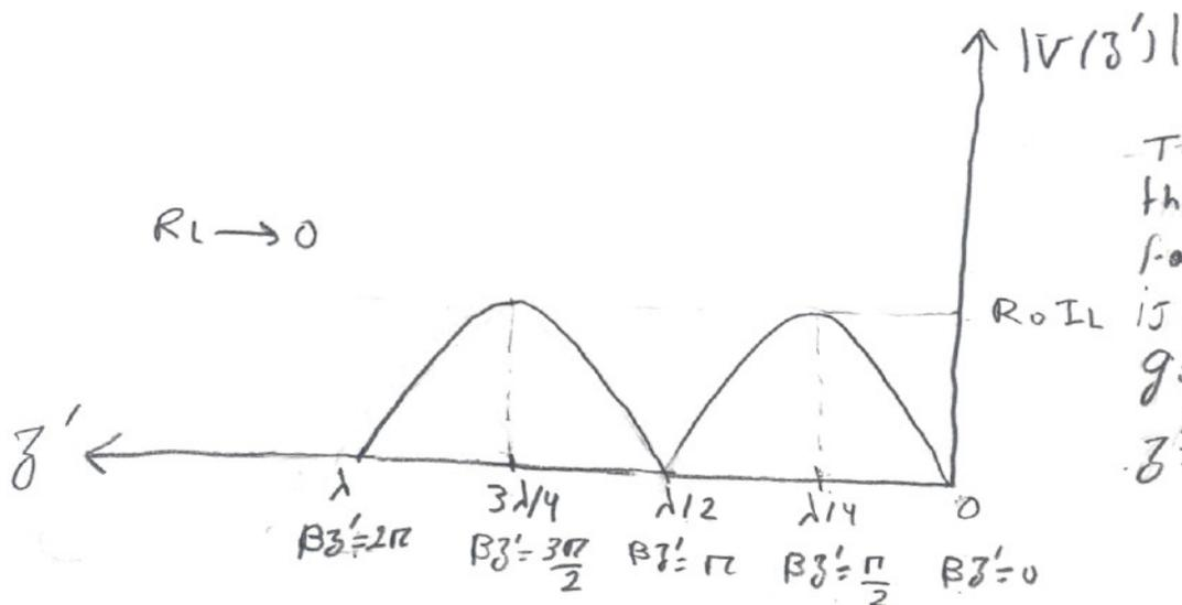
The difference between this curve & the one we found in class ( $R_L < R_0$ ) is that here  $|V(z')|$  goes to zero at  $z' = \lambda/4, 3\lambda/4, \dots$
