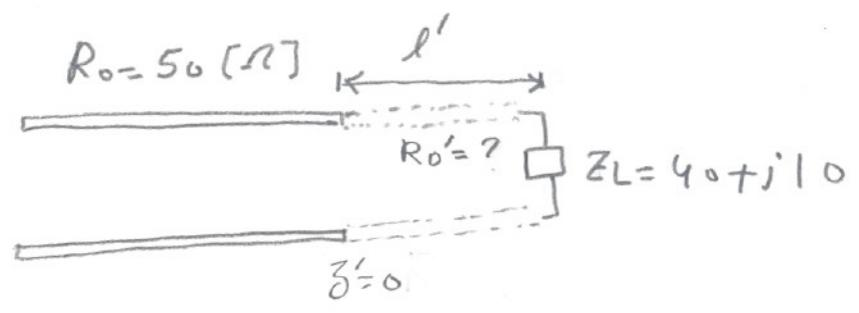
We calculate the input impedance seen at  $z' = 0$  & looking to the right (toward the load  $Z_L$ ). To have match condition this input impedance must be made equal to the original line impedance, i.e.  $R_0 = 50 \Omega$ .
