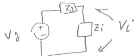
$$\textcircled{3} \quad V_i = V_g \frac{Z_i}{Z_i + Z_g} = 10 \angle 0$$
