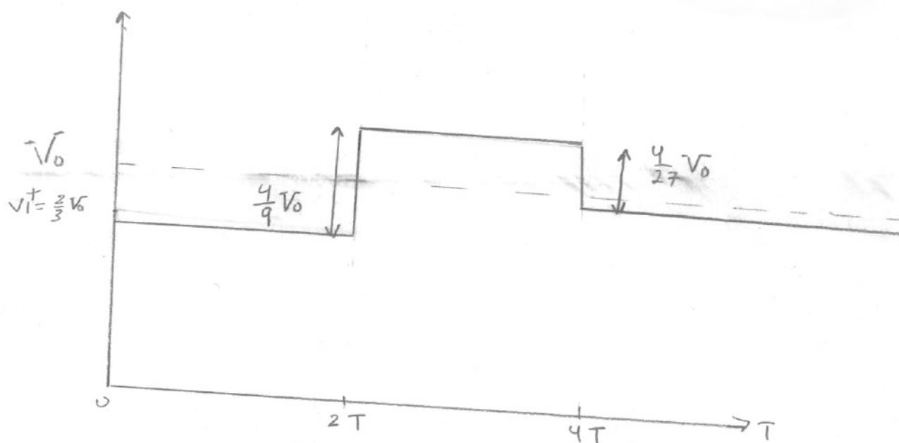
\* Note that Voltage goes above  $V_0$  for some time & drops below  $V_0$  at other time intervals, while it is approaching the value of  $V_L = V_0$
