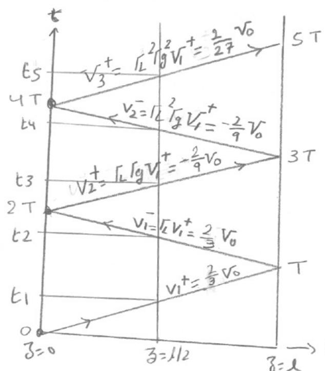
\* To find  $V(z=0, t)$  draw a vertical line at  $z=0$ . This intersects the directed lines at  $t=0, t=2T, t=4T, \dots$
