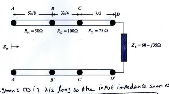
the segment CD is  $\lambda/2$  long so the input impedance seen at cc'is
