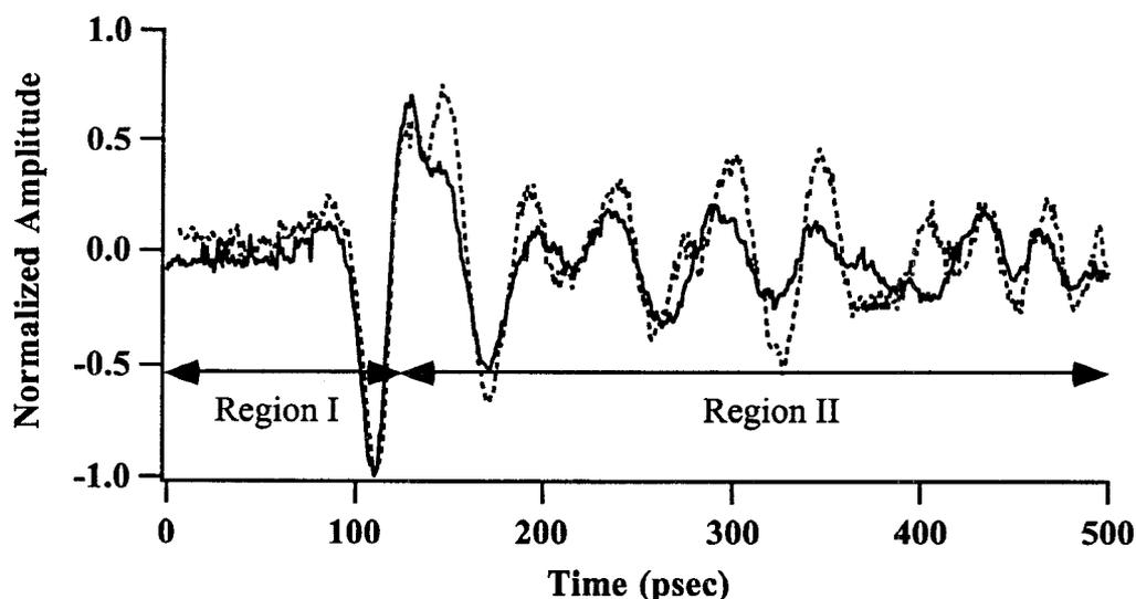
**Figure 4.** Response of the antenna that is in intimate contact with the M-crystal. The solid line is the reference and the dotted line is the M-crystal backed response. Region I is the pulse traversing through the LTG-GaAs substrate and Region II is the PC contribution.
