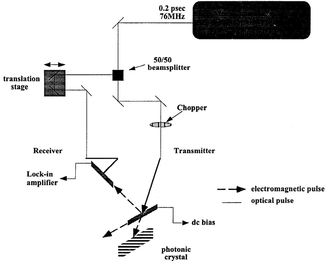
**Figure 1.** Experimental set-up used to photoconductively generate UWB electromagnetic bursts of energy. The transmitter is used in a broadside configuration to determine the effects of placing a substrate near the transmitter to reflect the energy that is radiated through the LTG-GaAs substrate.
