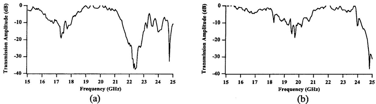
**Figure 2.** Frequency response of the component crystals in the UWB-PC. (a) The frequency response of the L-crystal and (b) the response of the M-crystal. The measurements are performed using a network analyzer sweeping from 15 to 25 GHz. The UWB-PC response is the superposition of the individual crystal responses.
