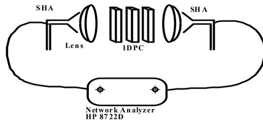
FIGURE 1. Frequency-domain experimental setup.
