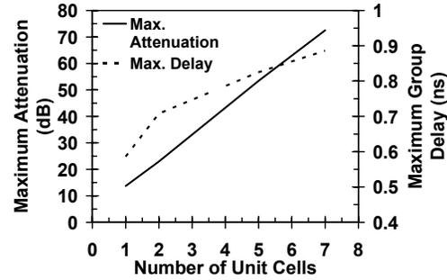
**Figure 4.** Negative group delay and attenuation as function of the number of SRRs and SWs.
