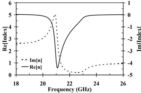
**Figure 1.** Real and imaginary parts of the index of refraction. The parameters used in obtaining figure 1 and figure 2 are  $\omega_{eo} = 0$ ,  $\omega_{mo} = 2\pi \times 21$ ,  $\omega_{ep} = 2\pi \times 40$ ,  $\omega_{mp} = 2\pi \times 23$  (GHz),  $\gamma_e = 2 \times 10^9$ , and  $\gamma_m = 10^9$  (1/s) respectively.
