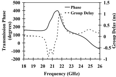
**Figure 3.** Transmission phase and group delay for a 7 element array of SRRs and SWs. The ring dimensions were scaled down from those in [2] for operation in the K-band. The strips are 0.2mm wide with  $\sigma = 5.8 \times 10^6 S/m$ .
