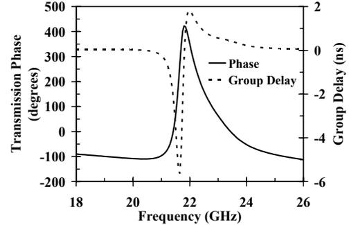
**Figure 2.** Calculated transmission phase and group delay for a 5mm thick LHM slab immersed in vacuum.
