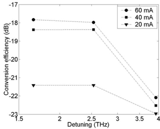
Fig. 4. Conversion efficiency as a function of frequency detuning for different injection currents.
