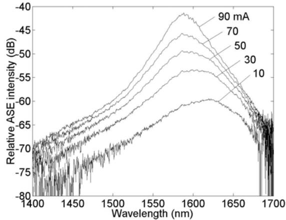
Fig. 1. ASE spectra taken at injection currents of 10–90 mA.
