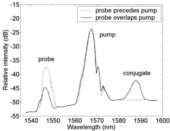
Fig. 3. Output spectra taken for two different delays between pump and probe.
