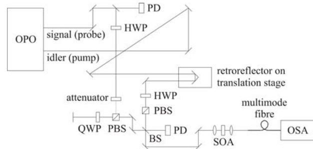
Fig. 2. Setup for the FWM experiment. OPO = optical parametric oscillator, PD = photodiode, HWP = half-waveplate, QWP = quarter-waveplate, PBS = polarizing beamsplitter, BS = beamsampler, OSA = optical spectrum analyzer.
