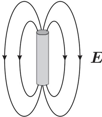
The answer is in a *capacitor*,  $\frac{V}{I} = (j\omega C)^{-1}$ . So, in the near field, this antenna is acting very much like a capacitor with the dipole 'ends' acting as plates giving a fringing capacitance.
