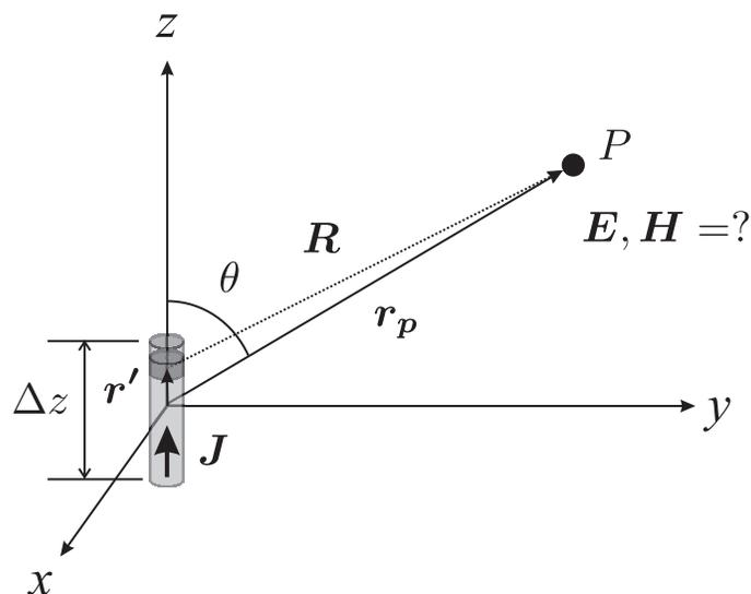
In this illustration,  $R$  is the distance from the current element to the field point  $P$ , and  $r$  is the distance from the origin to  $P$ .
