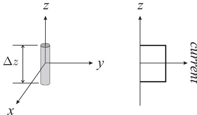
Although it is difficult to implement in practice (having a current distribution that is difficult to realize since it is discontinuous), it is highly useful for helping analyze larger wire antennas which can be subdivided into short sections having uniform current (i.e., ideal dipoles). Then, much in the same way as we derived vector potential for a continuous current distribution, we can use superposition to find the fields of a long wire antenna.
