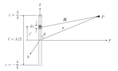
Now, since we are in the far field, the diagram above is not really correct. As the point P moves far from the source, the vectors  $\mathbf{R}$  and  $\mathbf{r}$  become parallel. This is known as the *parallel ray* approximation. Under this approximation,
