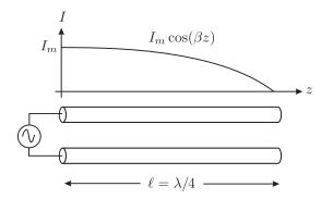
Note that there is no current at  $z = \lambda/4$  as required by the open circuit boundary condition. Now, if we "open" up the transmission line, we can essentially create a dipole that is half a wavelength long:
