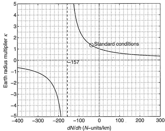
Figure 5: Plot of earth radius multiplier versus refractive index gradient
