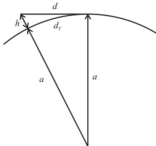
Figure 4: Link geometry
