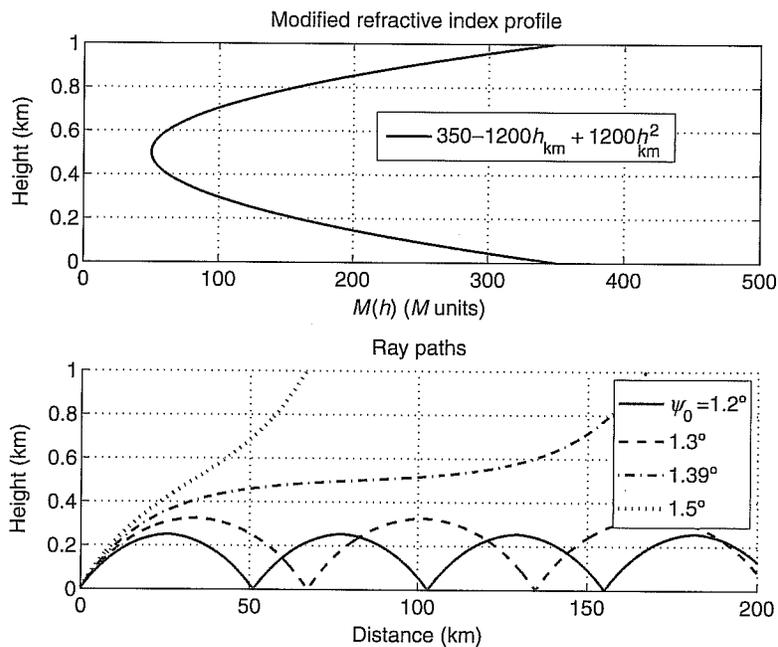
Figure 7: Ray-tracing calculations of ray trajectories for given atmospheric refractivity gradient
