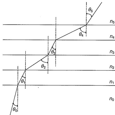
Figure 1: Stratified media representation of atmosphere
