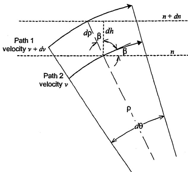
Figure 2: Ray bundle traversing the atmosphere
